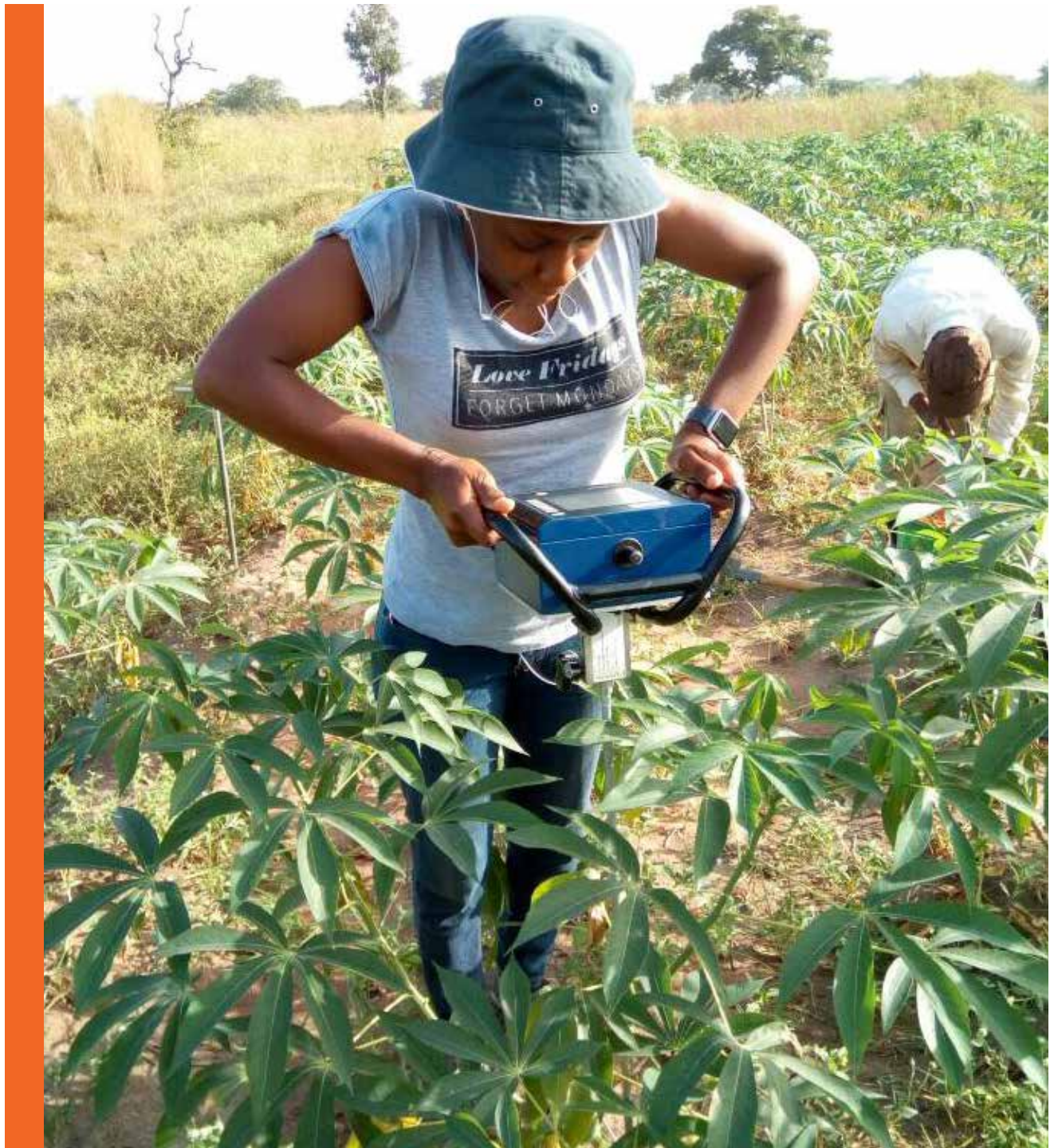
Omolara Olabisi, ACAI PhD student measuring soil resistance to penetration with penetrometer on a trial plot in Saki, Oyo State, Nigeria.
